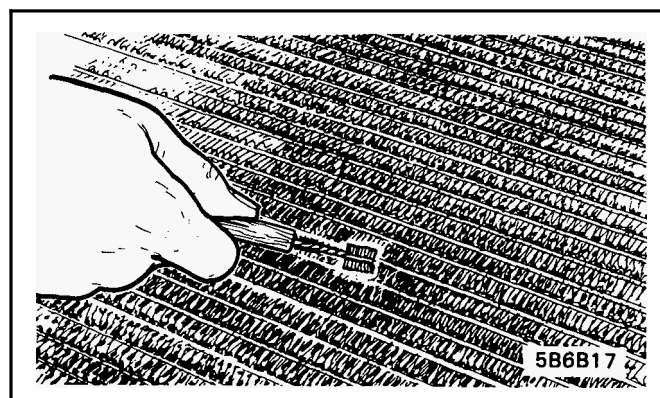
Figure 6B-22 Cleaning Area With Steel Brush
