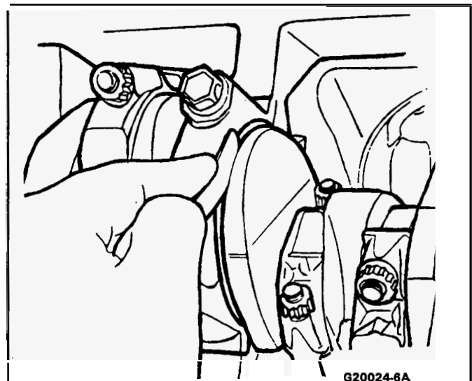
Figure 31 Measuring Crankshaft End Play
