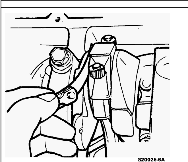
Figure 32 Measuring Connecting Rod Side Clearance (Single Rod Journal)
